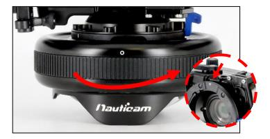
Turn the lens clockwise until the 'O' mark on the lens aligns with the WHITE dot on the converter and a "click" sound is heard
